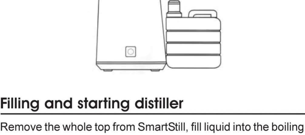
chamber. Do not fill above the filling line mark. Put the whole top
